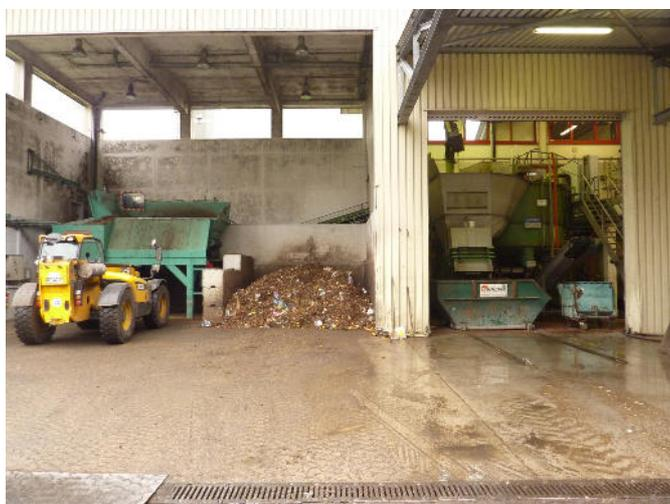
*Inlet station (left) and material pulper (right) of the IFBB processing.*
